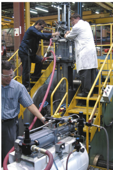
Members of Velan's Engineering Department conduct a test for an international architectural engineering firm of an automated valve to be used for turbine bypass isolation, a difficult power plant application.
