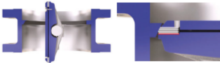
Figure 3 One of the benefits of using a wide gasket TOV is that it assures an even compression over the entire sealing surface of the bimetallic seal, resulting in a long seal life and tight shutoff.
