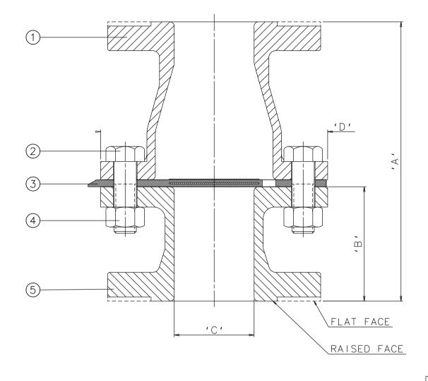
В С D Size(DN) 151 64.5 32 124 25 40 180 75.5 44 149 Component Material 198 80.5 57 162 50 BODY END CAST IRON 259 80 91 83 216 BODY/SEAT BOLT MILD STEEL DISK RUBBER 348 114 108 295 100
