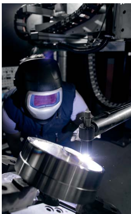
Body seats being welded.
