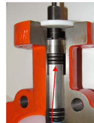
Live loaded secondary sealing
