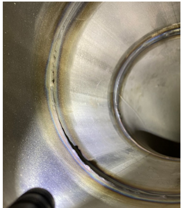
Burn-through or slag not ground smooth after welding
