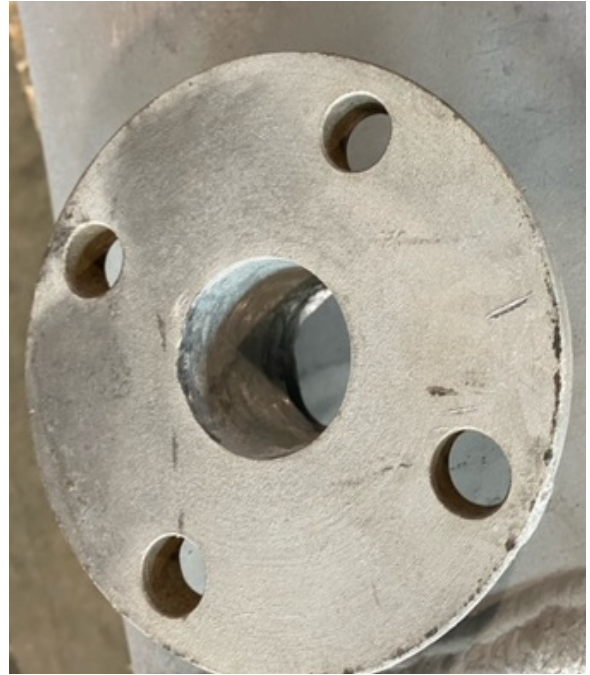
Burn-through or slag not ground smooth after welding
