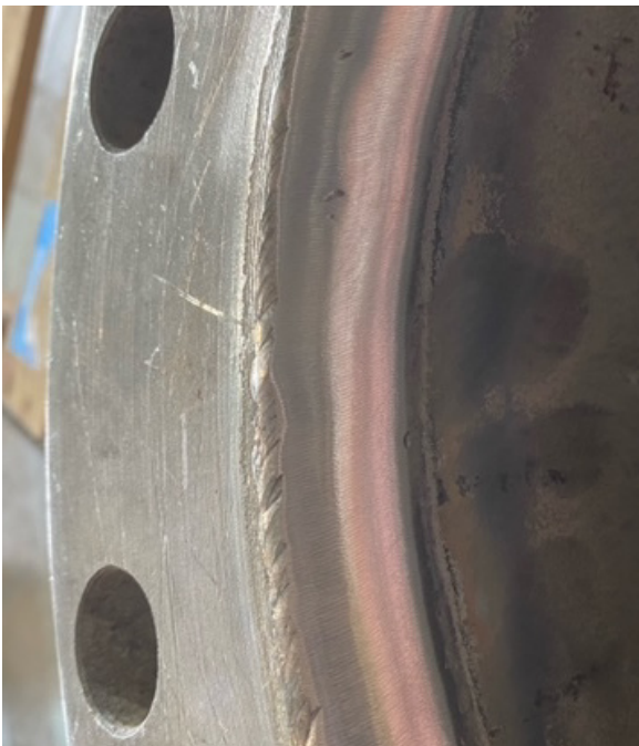
Flange face radius not ground / machined to appropriate radius
