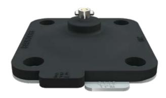
The Saunders® 214S/425 diaphragm features the Saunders® bayonet type compressor attachment which allows the diaphragm to float freely relative to compressor to avoid point loading of the PTFE at the stud. The bayonet fit also facilitates easy error free engagement of diaphragm and compressor.
