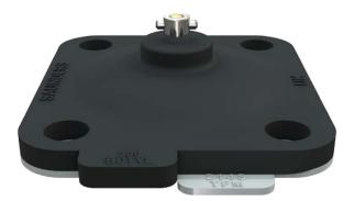
The Saunders® 214S/300 diaphragm features the Saunders® bayonet type compressor attachment which allows the diaphragm to float freely relative to compressor to avoid point loading of the PTFE at the stud. The bayonet fit also facilitates easy error free engagement of diaphragm and compressor.
