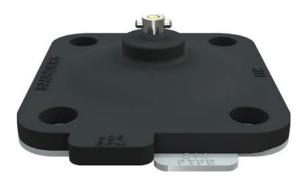
The Saunders<sup>®</sup> 214/425 diaphragm features the Saunders<sup>®</sup> bayonet type compressor attachment which allows the diaphragm to float freely relative to compressor to avoid point loading of the PTFE at the stud. The bayonet fit also facilitates easy error free engagement of diaphragm and compressor.
