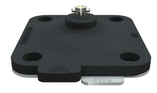
The Saunders® 214/300 diaphragm features the Saunders® bayonet type compressor attachment which allows the diaphragm to float freely relative to compressor to avoid point loading of the PTFE at the stud. The bayonet fit also facilitates easy error free engagement of diaphragm and compressor.
