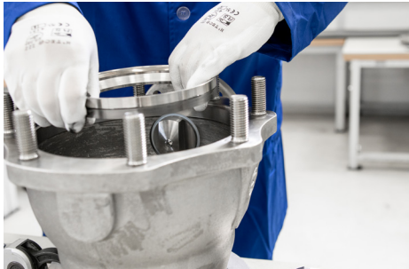
15. Insert seal ring (#40) over seat "B" (#6) and insert the two together into the valve cover or tail (#2). Apply grease to the sealing surfaces of the seat (#6). Apply pressure and axial force to pre-compress the seat seal according to the values shown in table B.
