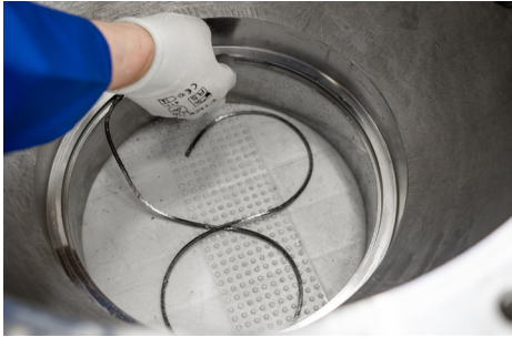
13. Insert wave spring (#41) into the Body part (#1).
