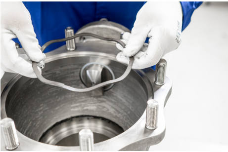
14. Insert S-ring (#42) into the body part (#1) over the wave spring (#41). Keep orientation of S-ring as shown in Fig.9.
