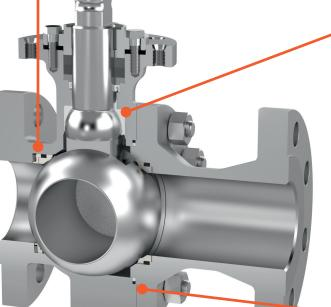
Alternatively, for higher temperature applications, Krombach offers a graphite packing arrangement with metallic diffusion barrier rings to ensure the highest levels of fugitive emissions containment without sacrificing LOW TORQUE OPERATION and Fire Safe protection.
