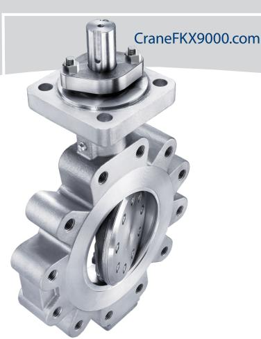
Torque-Seating: Unlike position-seated ball, butterfly or plug valves, the torque-seated Crane®FKX 9000 selfadjusts to evenly distribute seal compression. A "floating" seal ring and wide seal ring supporting gasket yield a BETTER SEAL to eliminate binding and to enhance performance.
