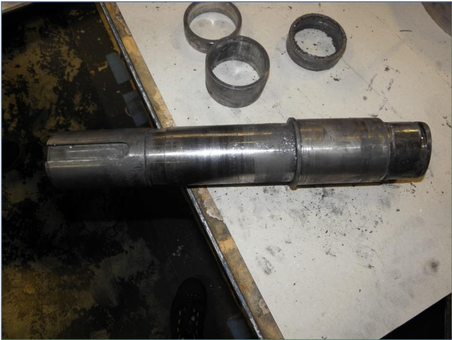
Photo 2: Stem Sealing Area and Bushing
